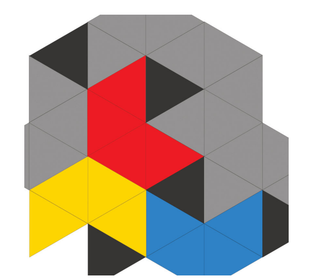
A section of the tessellation on the stainless steel cladding. The colours are intended only to show the way the chevrons fit around the triangles.
